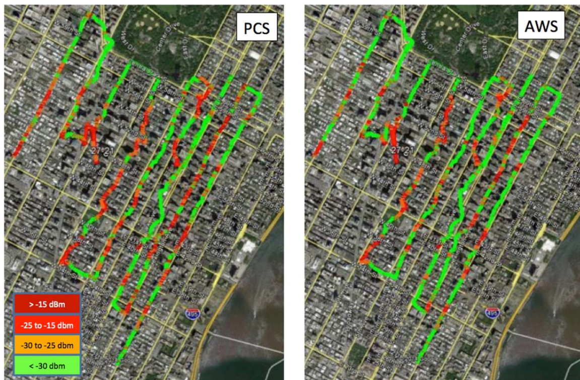
Figure 4: Distribution of very strong street level signals from T-Mobile in Manhattan
