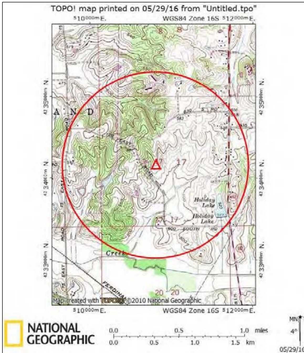
Figure 15. Visual APE for the Project Area (base map from Huntingsburg 7.5-minute Quadrangle). The triangle marks the proposed cell tower location with the circle establishing the Visual APE.
