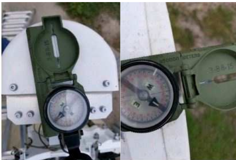
RSA/MDS verified the A Site and B Site Azimuths in Castle Hayne, NC.
